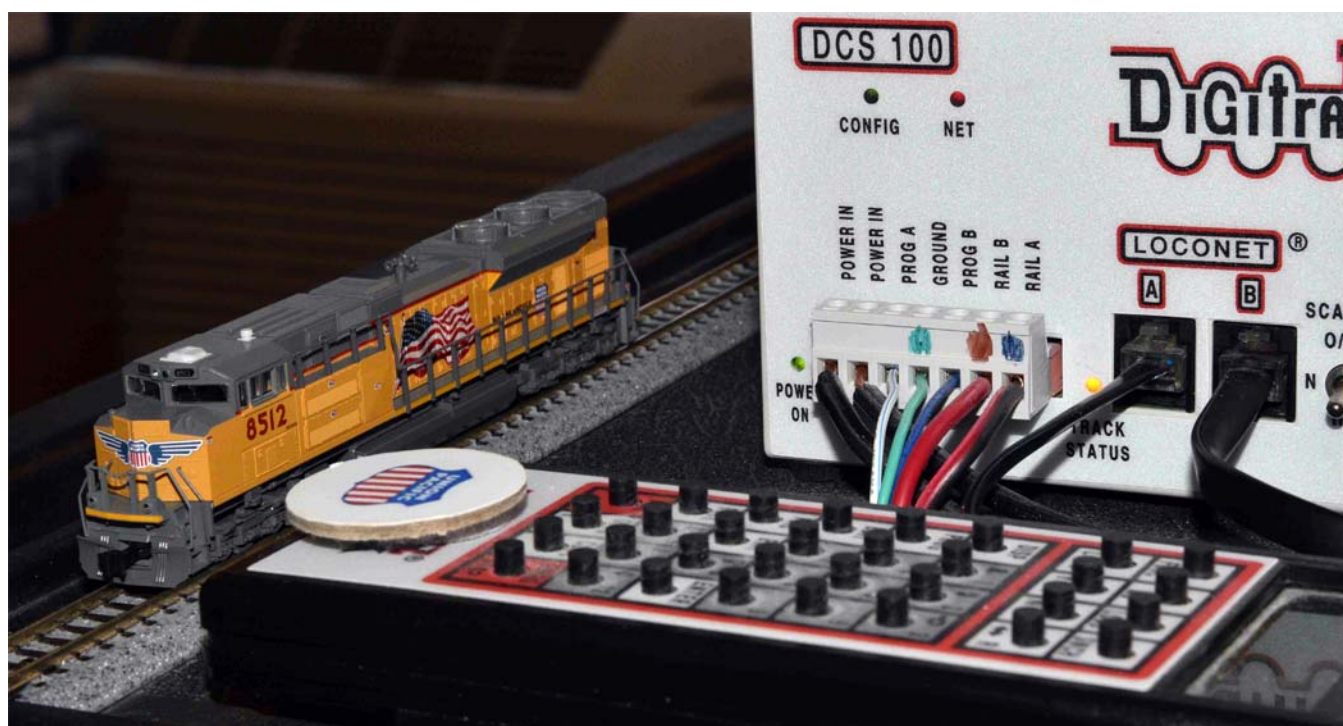
Newly-acquired Kato SD70ACe UP 8512 sits on Hugh Boyd's programming track awaiting setting of CV values for speed matching and headlight auto-dimming. Photo by Hugh Boyd.
